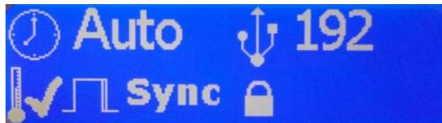
If the unit is locked to an external reference, **SYNC** is displayed on the bottom line. If an external reference is connected but the unit cannot lock to it or is in the process of locking to it, **SYNC** is displayed greyed out.
