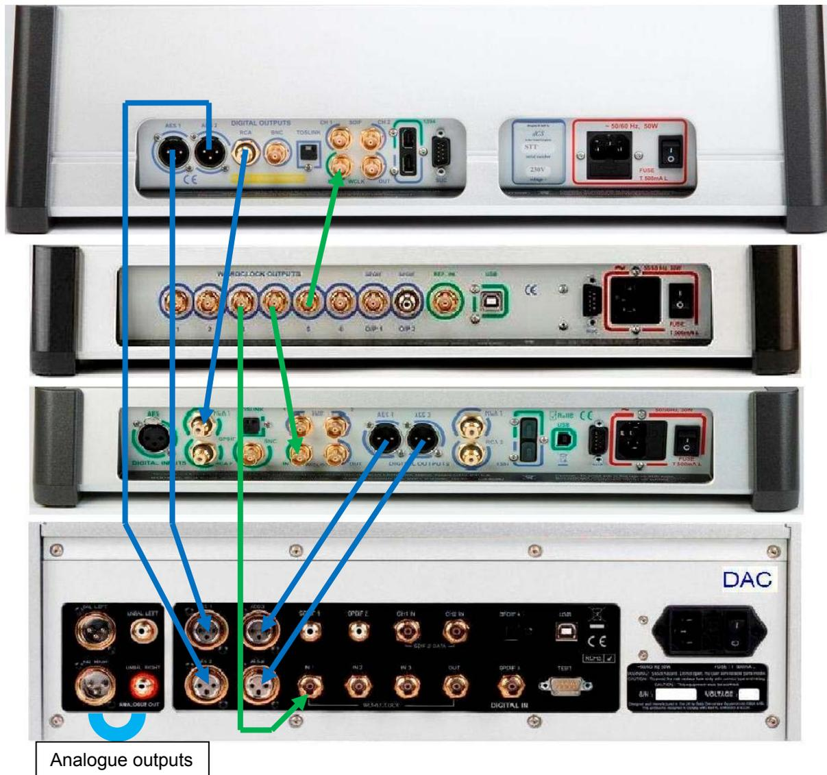
Figure 6 – Using a *Vivaldi* DAC with a *Scarlatti* stack
