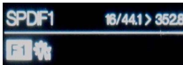
If the Upsampler is receiving a data stream in which the **NonAudio** flag has been set, the Upsampler will mute and display for example: **NA/44.1>DSD**. The Vivaldi Transport (v1.10 or later) sets the NonAudio flag when the CD tray opens and returns to Audio mode when playback starts.
