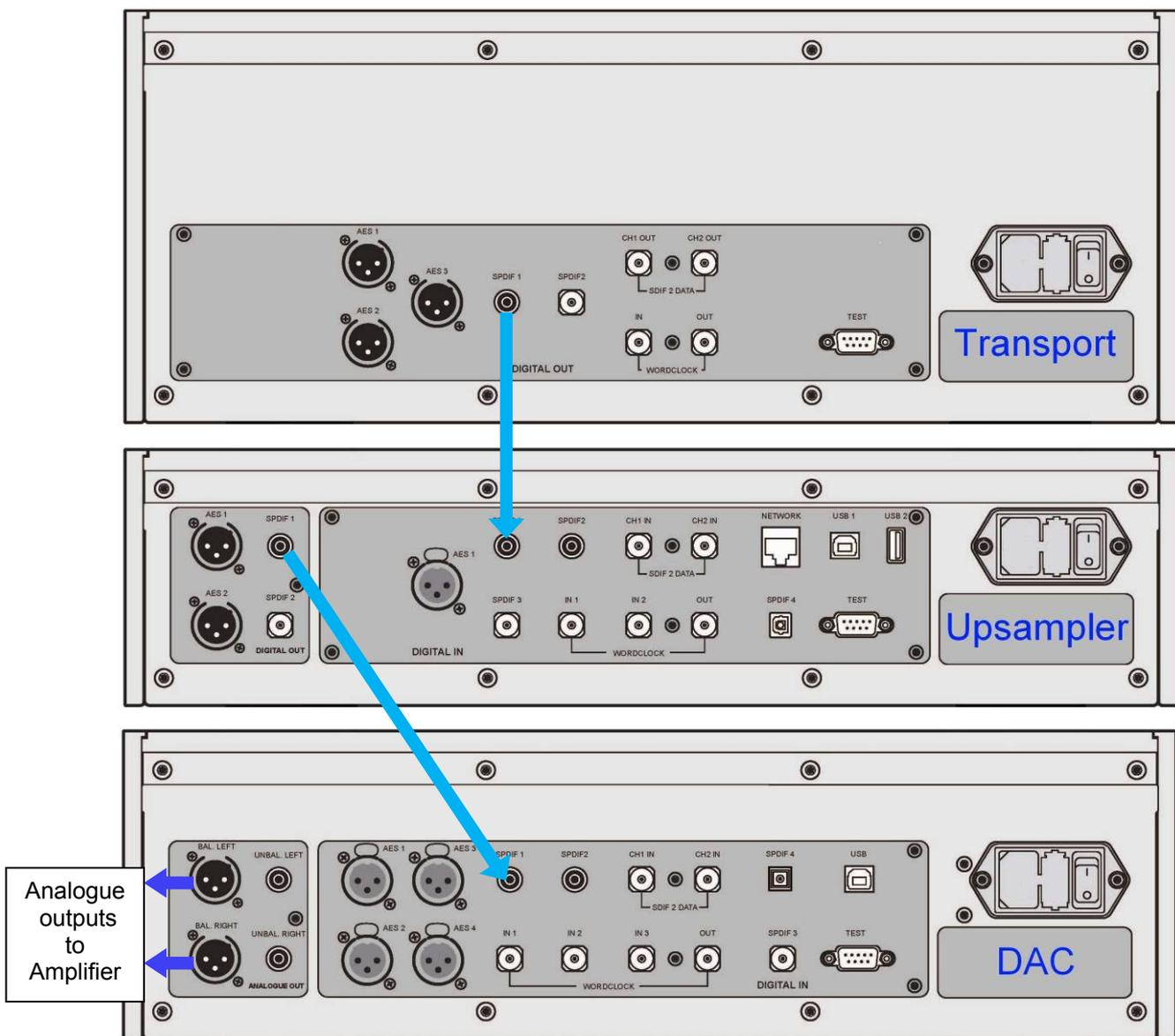
Figure 2 – Connecting a single-wire SPDIF output
