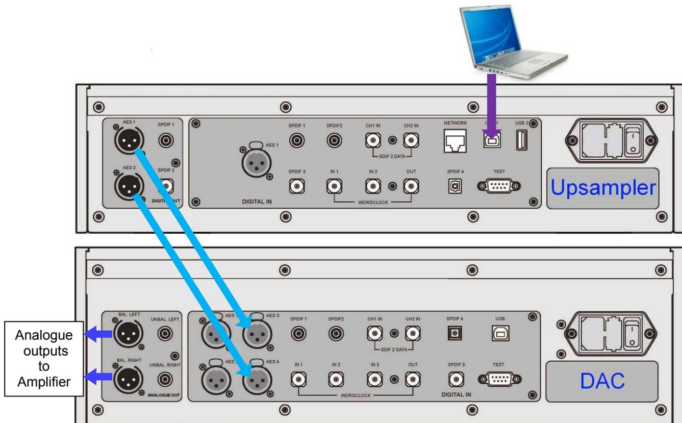
Figure 4 – Using a Vivaldi Upsampler and DAC with a laptop
