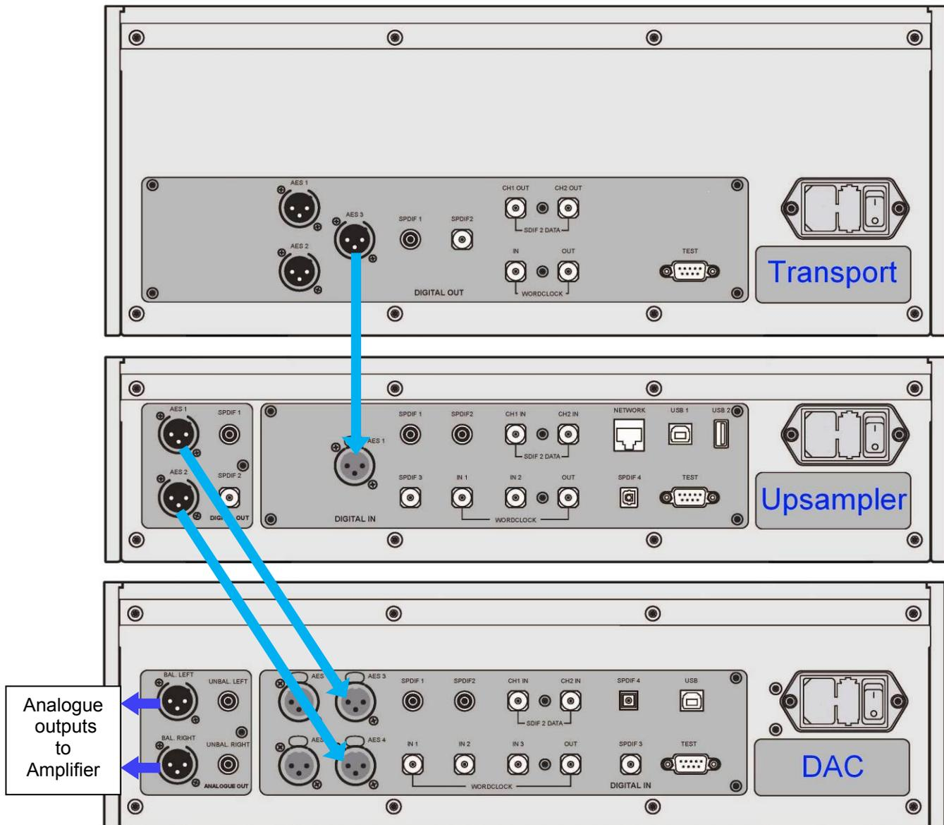
Figure 1 – Connecting the Dual AES output
