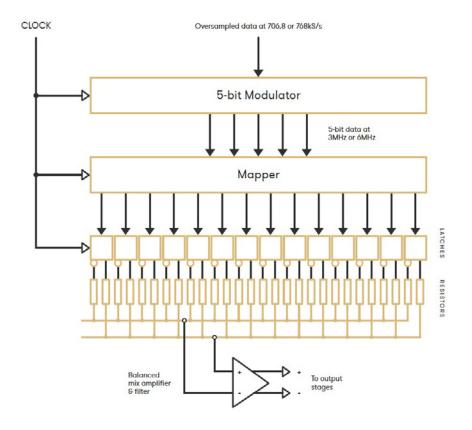
This diagram illustrates the basic layout of the Ring DAC
