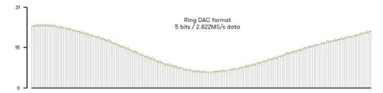
This diagram illustrates the output of the Modulator within the Ring DAC, modulating incoming digital audio signals to a 5-bit high rate format ready for conversion to analogue
