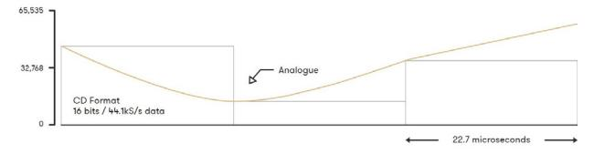
This diagram shows how an analogue sound wave can be represented with 16-bit 44,100 samples per second PCM encoding
