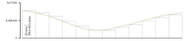
This diagram shows how an analogue sound wave can be represented with 24-bit 176,400 samples per second PCM encoding. The sample rate being higher than CD audio above allows for a greater representation across the X axis of this graph, whereas the higher bit-depth allows for the exact amplitude of the wave to be more accurately represented with each sample – the Y axis.
