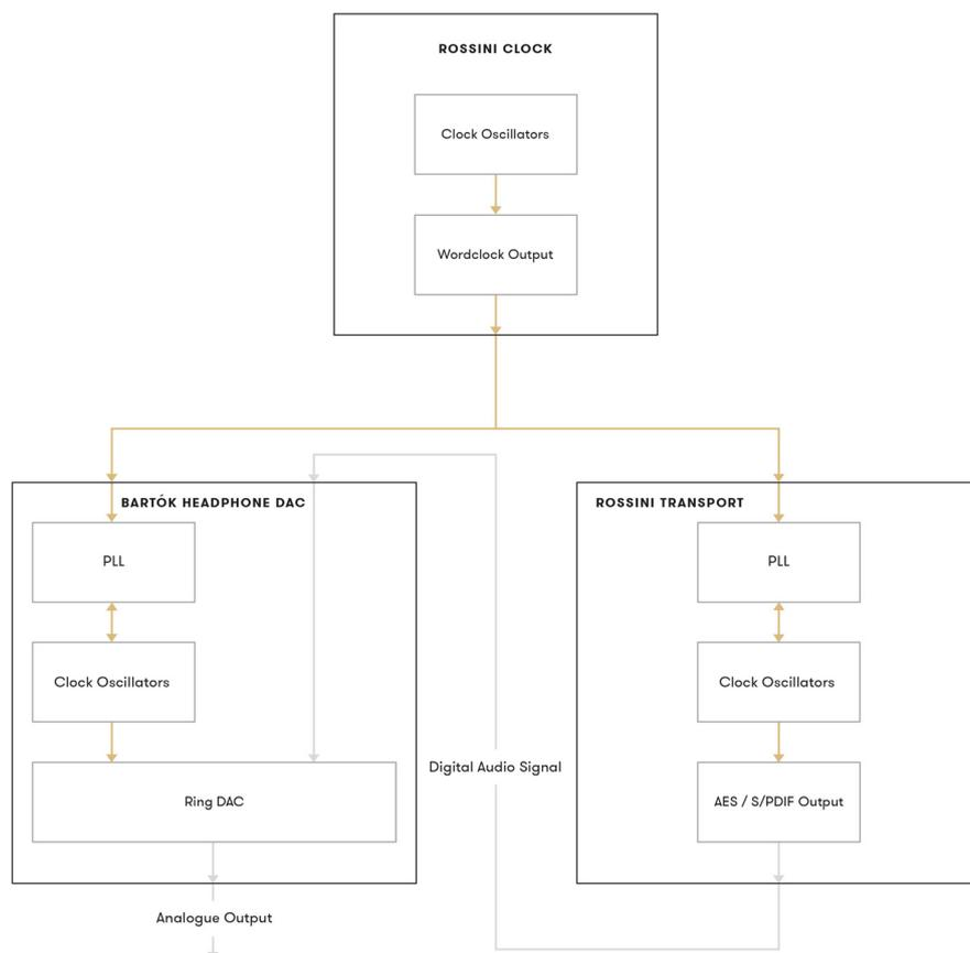
*This diagram shows an example of how a digital source (a Rossini Transport), a DAC (the Bartók Headphone DAC) and a master clock (the Rossini Clock) work together. The overall performance of the system is reliant on each of these stages performing correctly – each oscillator, PLL and output stage needs to operate at a high level to achieve optimum performance.*
